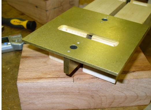
TJ-SR680 is designed to be used with a plunge router, a 3/4" OD guide bushing, and a 1/2" carbide router bit.
