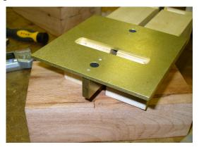
TJ-SR638 is designed to be used with a plunge router, a 1/2" OD guide bushing, and a 5/16" carbide router bit.
